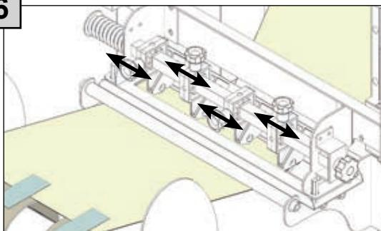
Position the blades in between each column and on either edge if desired.
