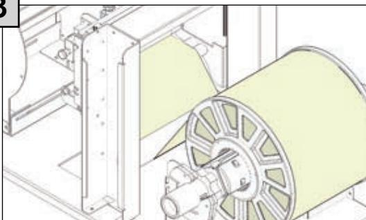
Guide the media under the first roller and use the picture below for the media path.
