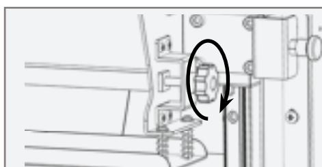
The black knobs lock the slitter module in the requested position.
