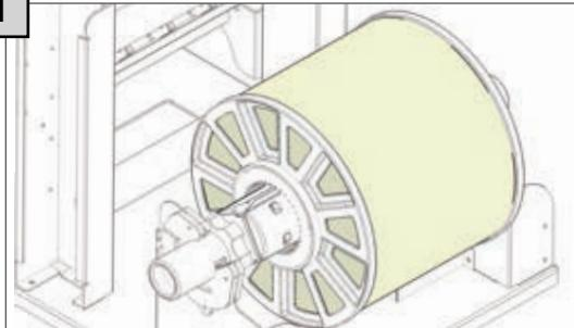
Insert the unwinder core holder onto its respective support.
