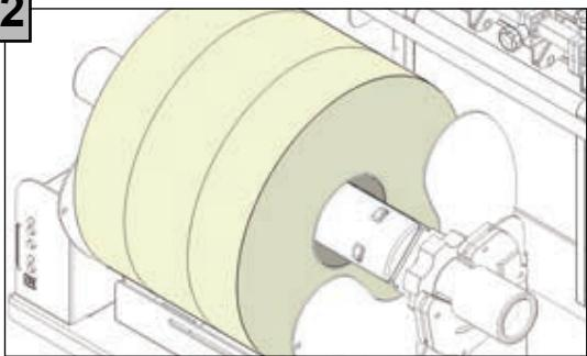
When the roll is finished, the unit automatically stops.
