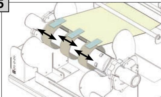
Temporarily attach the label directly to the take-up core holder.
