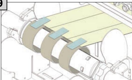
Make sure the tension on all rolls is even and attach each label to the core using a waste label.
