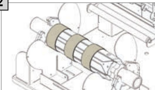
Insert the rewinder core holder onto its respective support.
