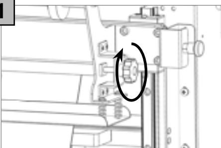
Remove the iron bar by unscrewing the black thumb screw.
