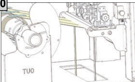
Allow the trimmed waste edges to fall into the waste basket under the hole.
