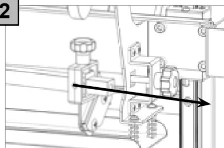
Insert or remove the blade holder(s) depending on the job.
