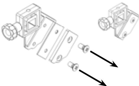
Loosen the two screws holding the blade in place.
